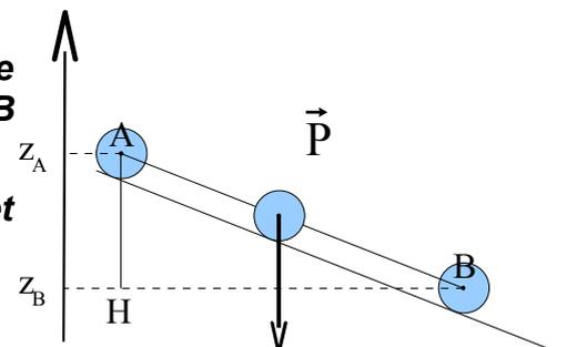
$$W_{AB}(\vec{P}) = \vec{P} \cdot \vec{AB} = P \times AB \times \cos \alpha = P \times AH = mg(z_A - z_B)$$
